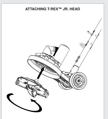
To attach the head, place the center piece of the head on the threaded piece located underneath, at the center of the T-REX $^{\text{TM}}$  Jr. Once on, twist counter-clockwise.
