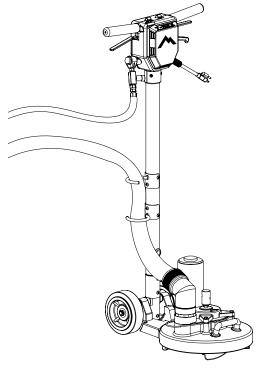
Connect solution hose from your extractor to swivel QD fitting on T-REX $^{\text{TM}}$  Jr. handle. Also, connect vacuum hose from extractor to Clear View Cuff-Lynx $^{\text{TM}}$  elbow or A105 lead hose.
