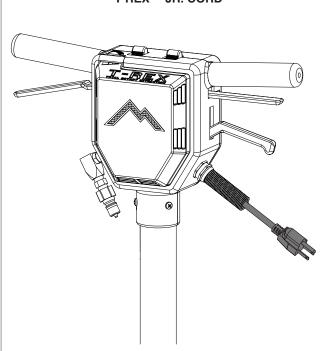
Connect pigtail plug to 25' power cord. Plug power cord into a grounded wall outlet.
