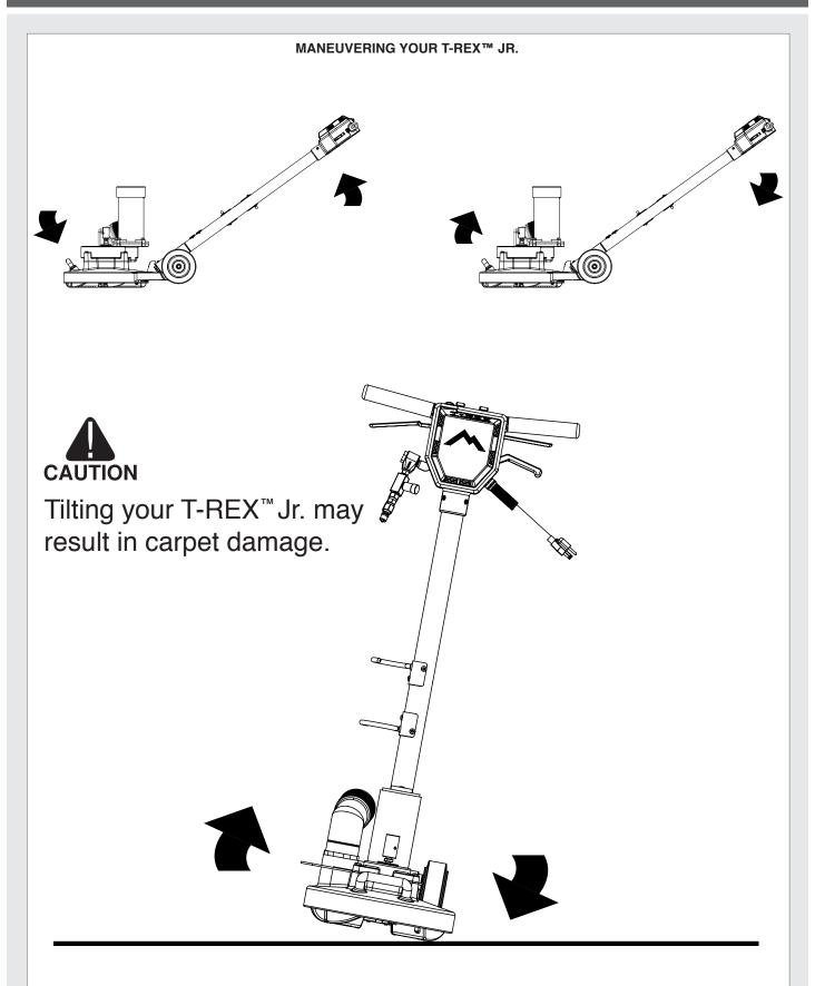
Your T-REX™ Jr. maneuvers much like a floor machine. Slightly lift handle to move to the right. Press the handle down slightly to move to the left. Tilting your T-REX™ Jr. may result in carpet damage. Remember to always keep T-REX™ Jr. evenly balanced on the surface.
